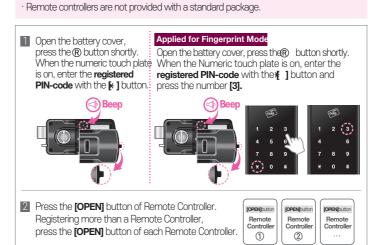
▶ To synchronize the password between the door lock and the remote control, you must press the button of the remote controller at least 3 times when using it for the first time, and after that, press once to open the door. When replacing the door lock battery, the remote control must be expected. the remote control must be synchronized.
